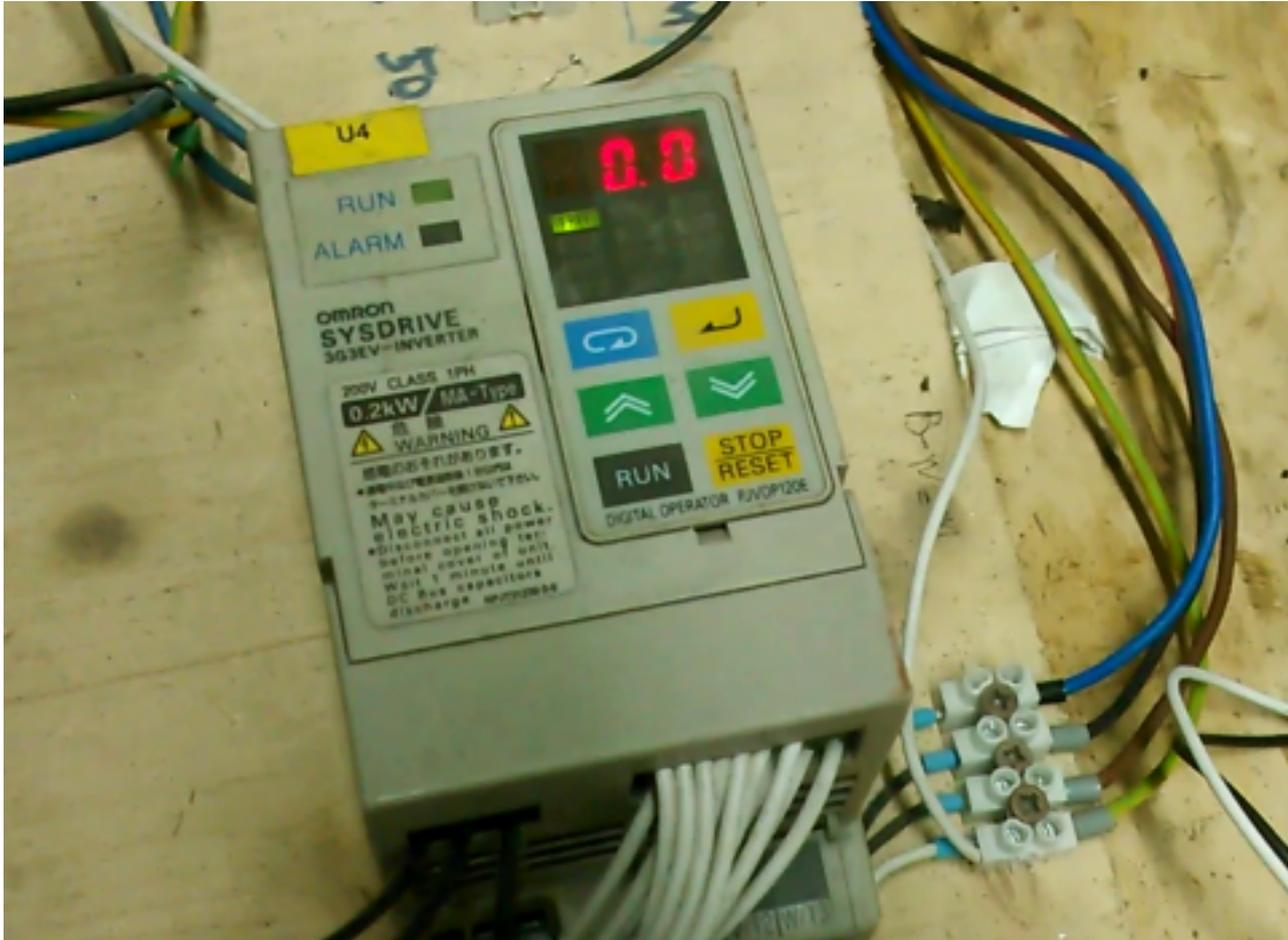
Inverter Omron modello Sysdrive 3G3EV
